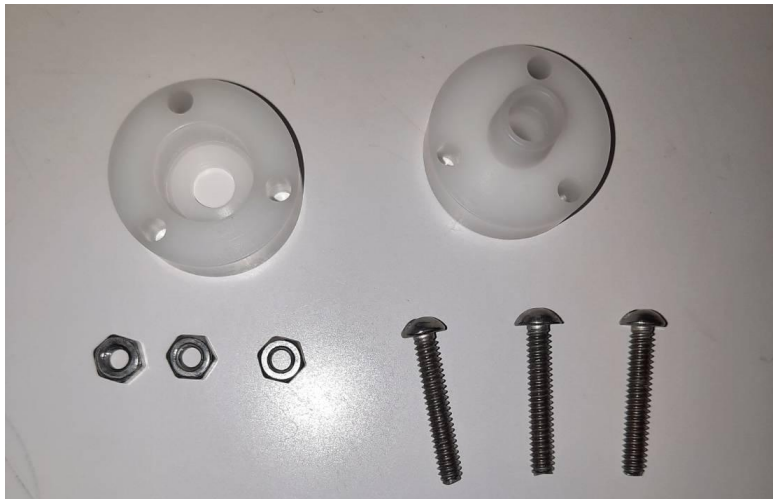
Figure 1. MatTek Permeation Fixture (EPI-200-FIX) parts. Parts include a top piece with protruding annulus (tube) and bottom piece with a chamber, along with 3 screws and nuts.
