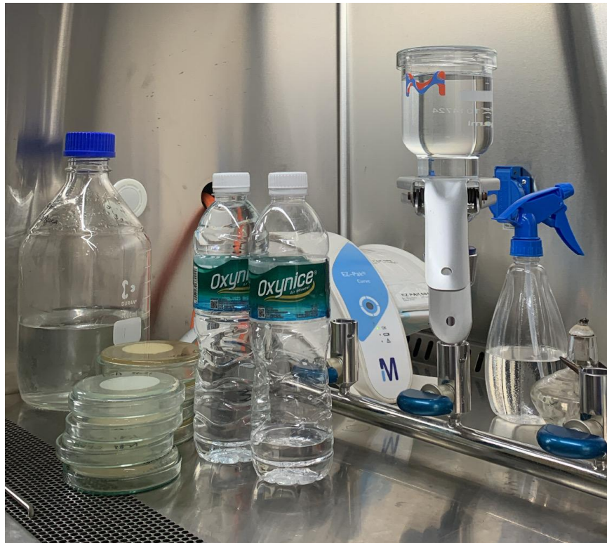
Appendix 8. Membrane filtration apparatus in BSPJI's microbiology laboratory
