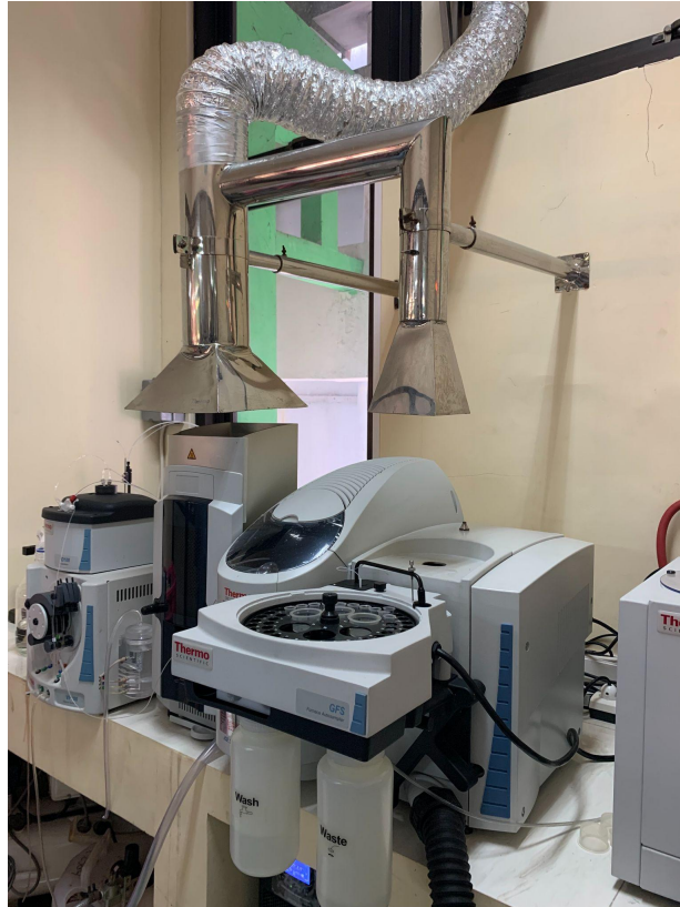
Appendix 3. Graphite furnace Atomic Absorption Spectrophotometer (AAS) used in BSPJI
