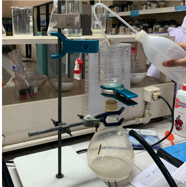
Appendix 5. Total Suspended Solid (TSS) analysis in BSPJI's environmental-chemistry laboratory
