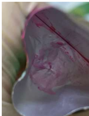
Figure 20. Crack Aluminium Foil (CA)
