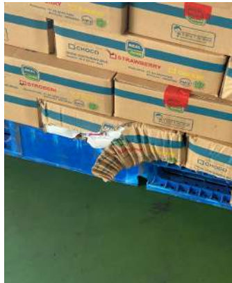
Figure 23. Torn corrugated fibreboard
