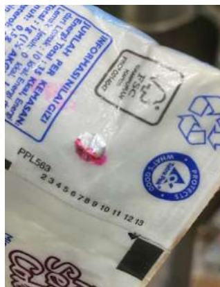
Figure 22. Crack straw hole (CS)
