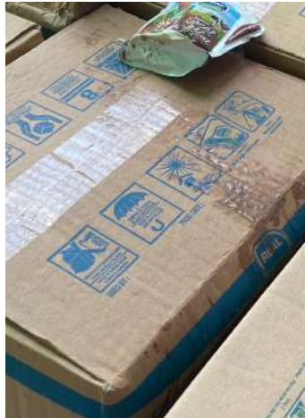
Figure 25. Wetted corrugated fibreboard by leak content of the product
