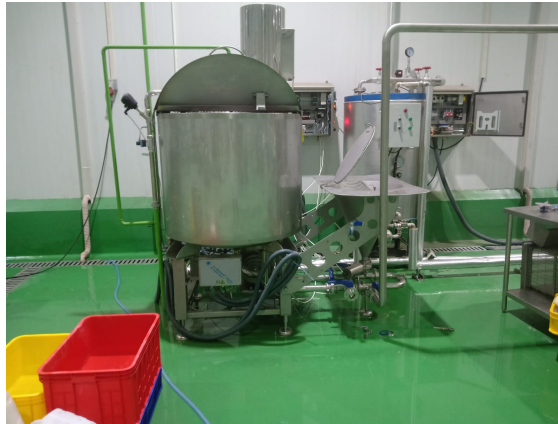
Figure 5. Feed Tank of the Injection Machine
