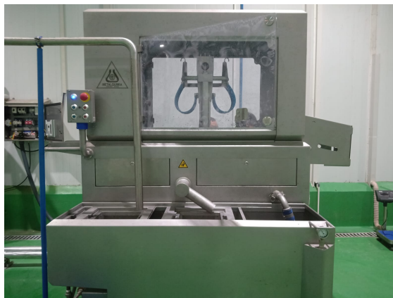
Figure 6. Injection Machine Used to Make Meltique Meat.
