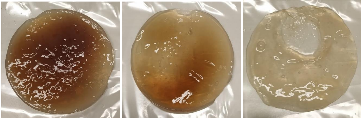
Appendix 3.1. Physical appearance of BC biofilms produced at different initial molasses concentration. From left to right: produced at 10%, 15%, and 20% (w/v) molasses concentration
