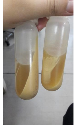
After 24 hours of mixing with rotator, the suspension was centrifuged and supernatant was collected
