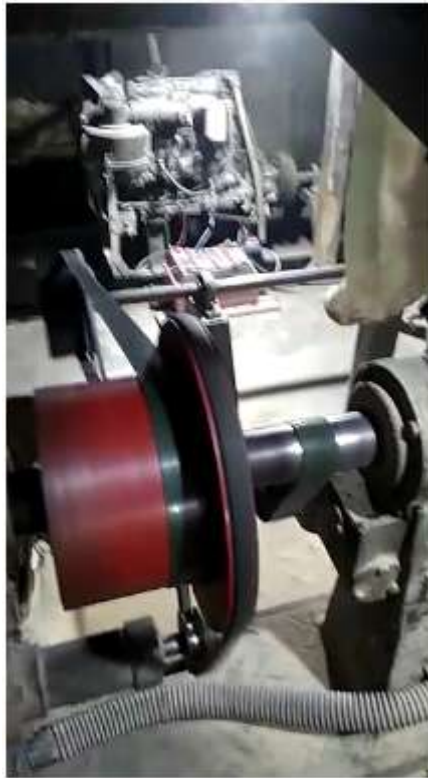
Figure 29. Belt and pulley that connect the machine and the engine
