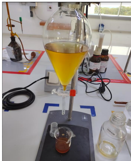
Figure 6. The biodiesel in a separating funnel to separate the biodiesel from glycerin
